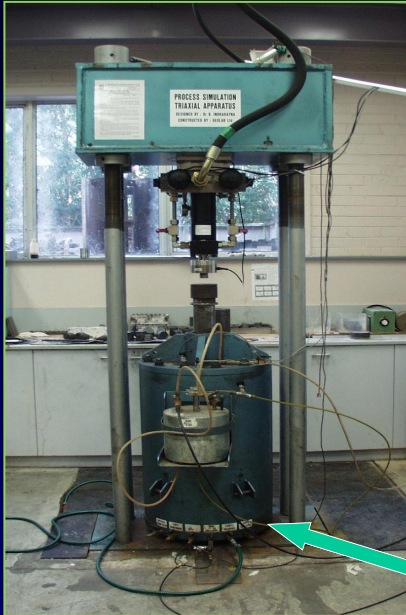
Cylindrical Triaxial Equipment (Specimen: 300 mm dia.x600 mm high)
