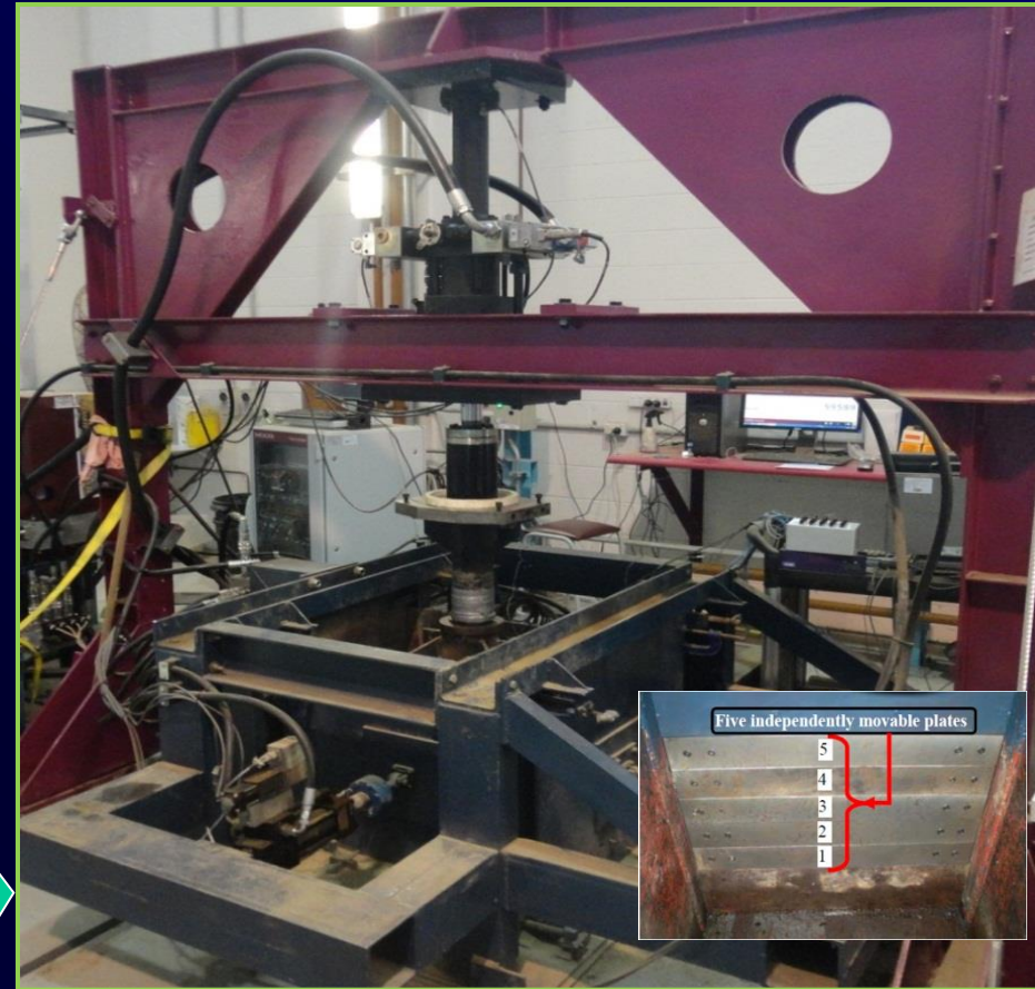
Prismatic Triaxial Rig to Simulate a Track Section (Specimen: 800x600x600 mm)
